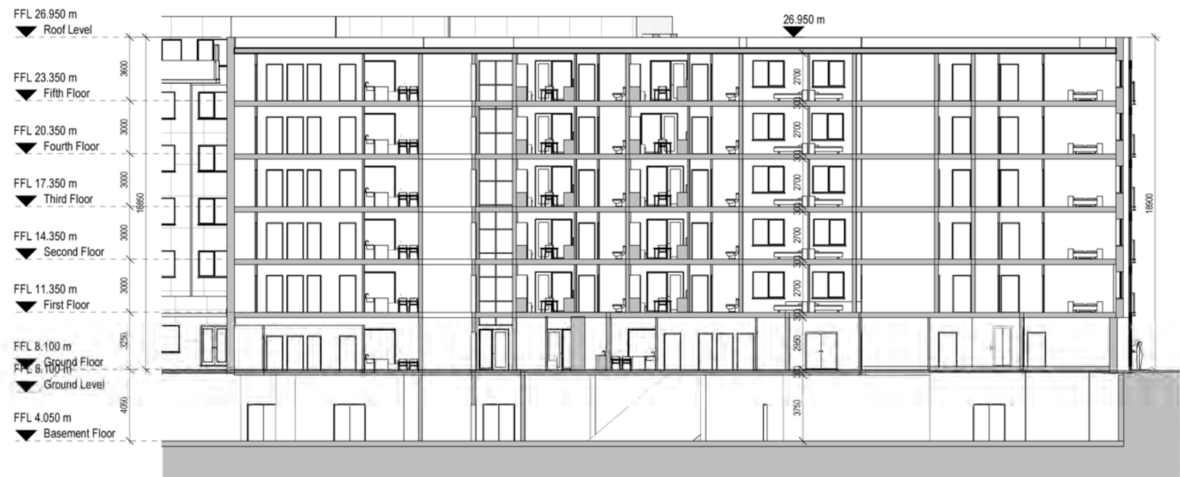
Block A Section B-B
